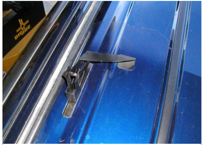
Receiver installed on roof
