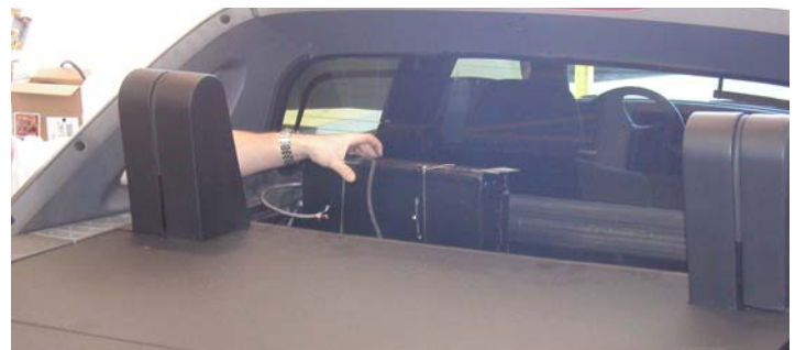
Carefully lower pump box and switch into the bed
